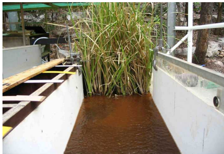
Fig 2. Zone of backwater upstream of the Vetiver buffer strip
